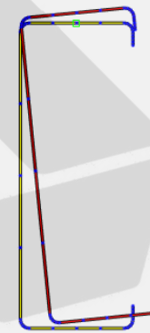
Buckled shape for CUFSM results
